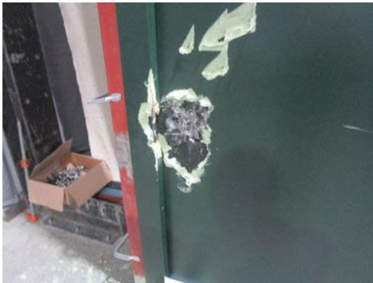
Photo No. 4 Final Condition of Lock Side Location of Inswing Door (Attack Side)
